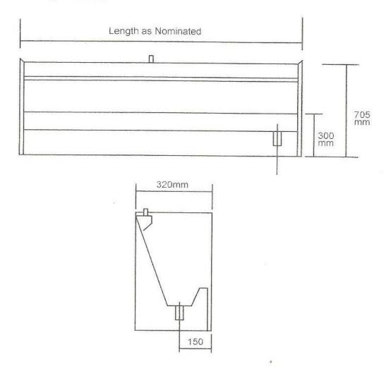
Material Commercial grade 1.2 304 stainless steel / 316 grade on request 50mm Left & Right Hand Outlets
